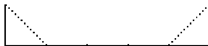
Phase 1 - Set out the baseline and triangulate two points offset 20m from the ends
