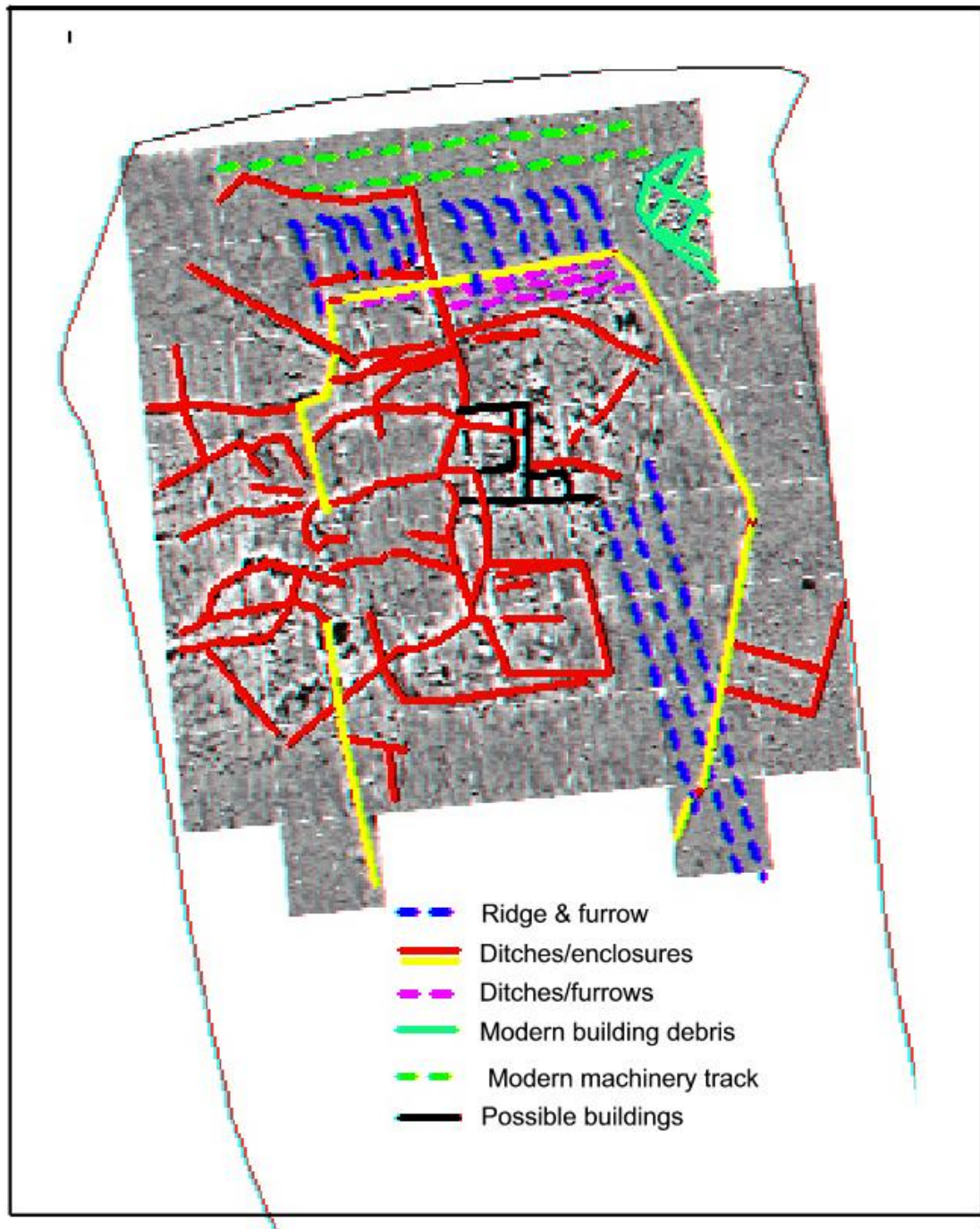
Fig 4 Interpreted plan of gradiometer survey results
